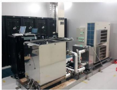
Satsuki Configured with 20 bricks instead of normal 16 computation bricks First TOP500 Supercomputer operated in a PRIVATE OFFICE
